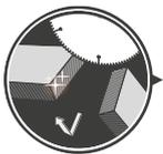
**PERFECT SURFACE** - Special teeth geometry optimal for high-performance batch cutting of strips and small-size elements guarantees a very high cutting quality and a perfect surface material cut.
