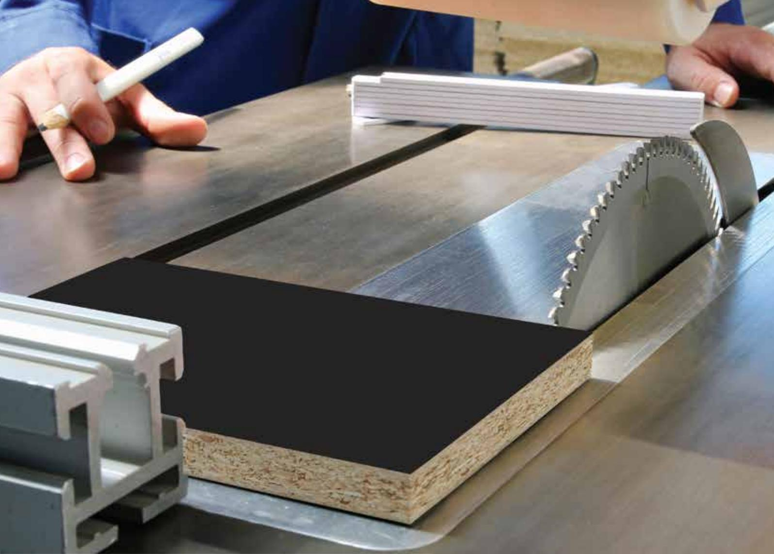
The new series are equipped with super hard NANOGRAIN carbide with a hardness of 2.250HV (series LL CUT VH line) and ULTRAFINE with a hardness of 2.100HV (series LL CUT line).
